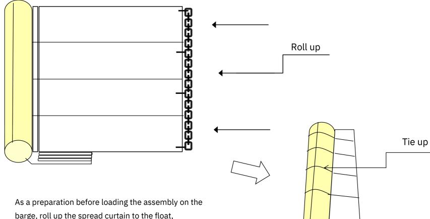
barge, roll up the spread curtain to the float, and tie the float and curtain together by using pp rope, approximately 10mm diameter, 5m length
